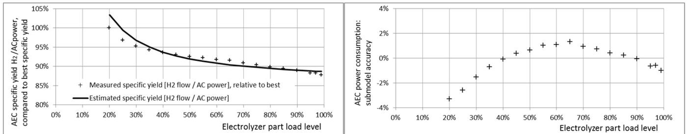
**Figure 2 Left:** AEC specific yield [H<sub>2</sub> produced / AC power consumed] relative to best operation point, model vs in-situ measurements. **Right:** Optimization model accuracy on AEC unit AC power consumption.
