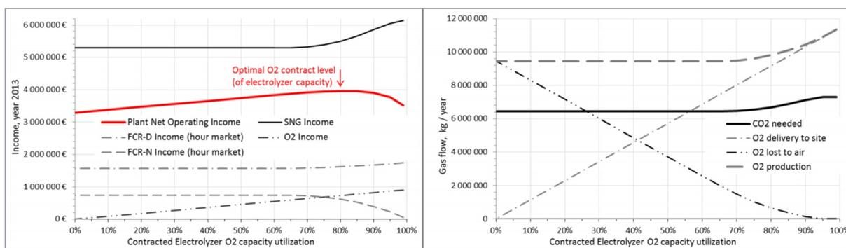
**Figure 3 Impact of contracted O<sub>2</sub> level on plant net operating income (left) and on CO<sub>2</sub> needed and O<sub>2</sub> produced, delivered or lost (right)**
