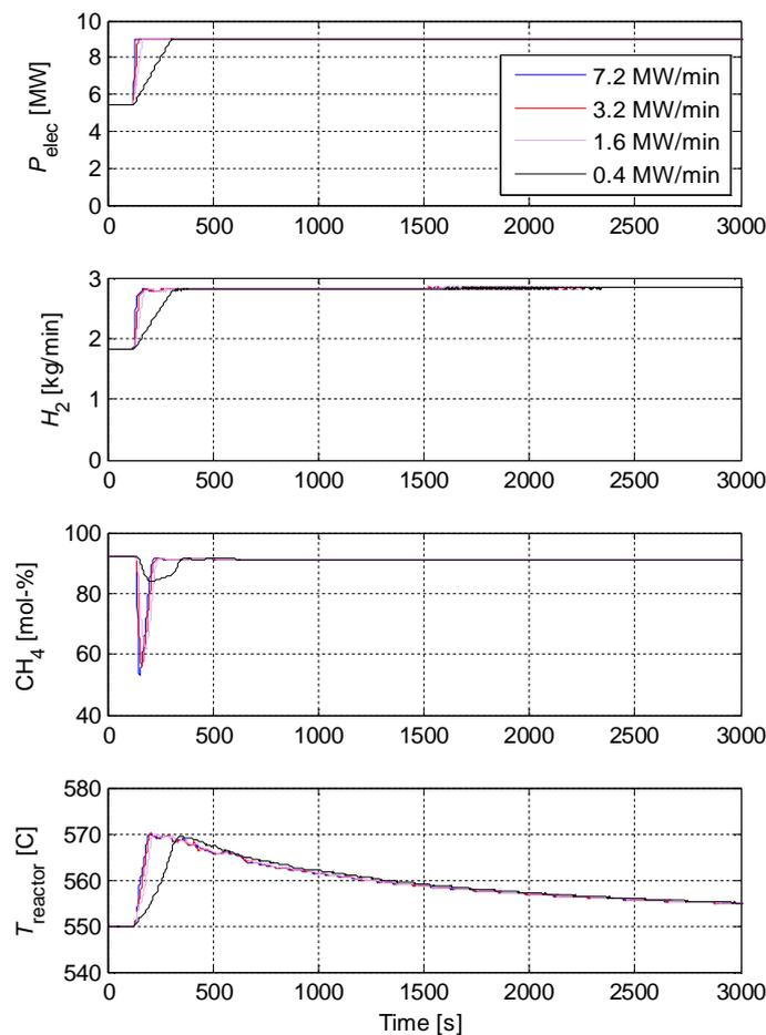
Figure 4. Ramp responses of the reference 9 MWe PtG plant.
